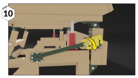
Secure the table with the new yellow clips on both sides.
