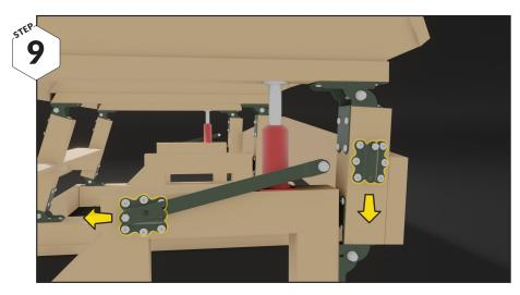
Place the clip holders in their new position acording to the yellow clip positioning. (see assembly instructions for Table kit 80320)
