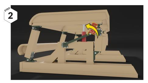
Remove the red clips on both sides.
