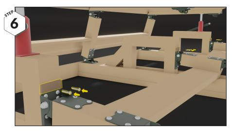
Screw a 15mm thick hardwood board on each pillar.
