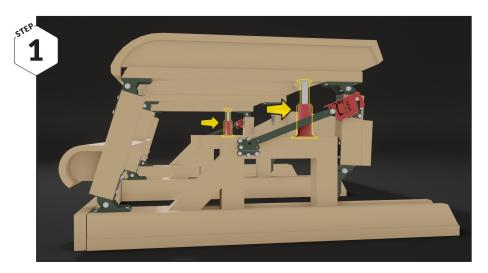
Secure the top part of the fence using car jacks or similar.
