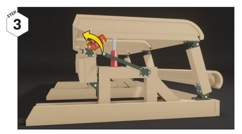
Remove the red clips on both sides.
