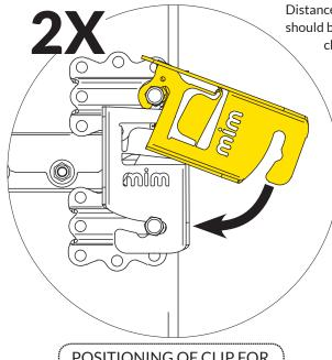
Distance between brackets should be adjusted to avoid clip C rattling.
