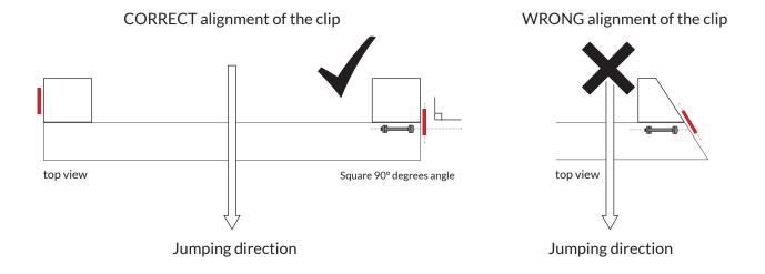
The **C** pieces must be: 8X - 90°(±10°) HORIZONTALLY LEVELLED not included DISTANCE BETWEEN C PIECES M-TS10X90 2X 0) The **C** pieces must be: PARALLEL AND HORIZONTALLY LEVELLED
