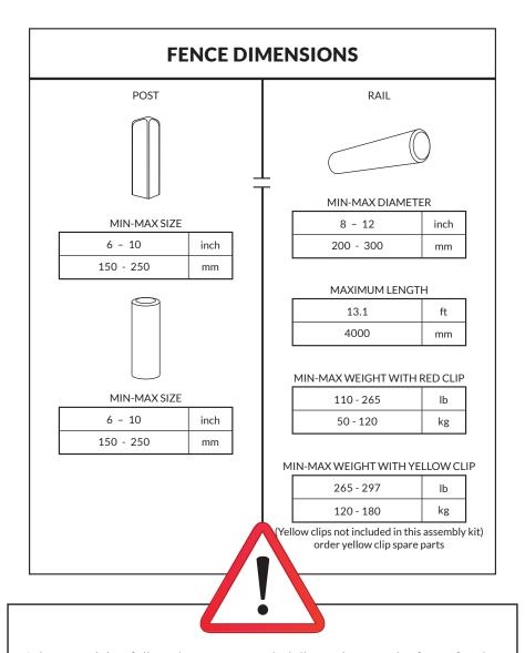
It is essential to follow the recommended dimensions on the fence for the correct function. If the recommended procedure is not correctly followed it may cause the failure of the device.
